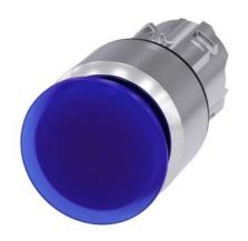
Illuminated mushroom pushbutton, 22 mm, round, metal, shiny, blue, 30 mm, latching, pull-to-unlatch mechanism, with laser labeling, symbol number according to, ISO 7000 or IEC 60417
