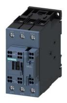
Traction contactor, AC-3 80 A, 37 kW / 400 V 1 NO + 1 NC 72 V DC, 0.7-1.25  $^{\circ}$  Us with varistor 3-pole, size S2 Spring-type terminals
