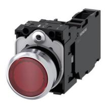
Illuminated pushbutton, 22 mm, round, metal, shiny, red, pushbutton, flat, momentary contact type, with holder, 1 NO+1 NC, LED module with integrated LED 24 V AC/DC, screw terminal, with laser labeling, upper case and lower case, always upper case at beginning of line
