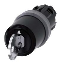
Key-operated switch IKON, 22 mm, round, plastic with metal front ring, lock number 360012K1, with 2 keys, 3 switch positions I-O<II, left latching, right momentary contact type, actuating angle 2x45°, 10:30h/12h/13:30h, Key removal O+I Z=50-unit packaging
