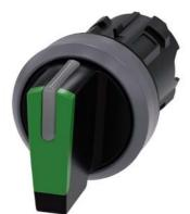
Selector switch, illuminable, 22 mm, round, plastic with metal front ring, green, selector switch, short, 3 switch positions I>O<II, momentary contact on the left, latching on the right, actuating angle 2x45°, 10:30h/12h/13:30h, with laser labeling, inscription or symbol Customer-specific selection with SIRIUS ACT configurator (CIN)
