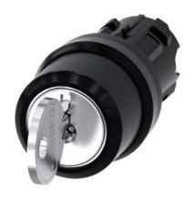
RONIS key-operated switch, 22 mm, round, plastic, special lock, with 2 keys, 3 switch positions I-O<II, left latching, right momentary contact type, actuating angle  $2x45^{\circ}$ , 10:30h/12h/13:30h, key removal O, possible special locks: SB31, 421, 455
