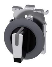
Selector switch, illuminable, 30 mm, round, Metal, matte, white, selector switch, short, front ring for flush installation, 3 switch positions I>O<II, momentary contact type, actuating angle 2x45°, 10:30h/12h/13:30h, with laser labeling, lower case
