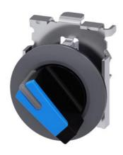
Selector switch, illuminable, 30 mm, round, Metal, matte, blue, selector switch, short, front ring for flush installation, 2 switch positions O-I, latching, actuating angle 90°, 10:30h/13:30h, Z=50-unit packaging
