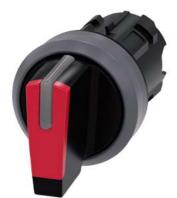
Selector switch, illuminable, 22 mm, round, plastic with metal front ring, red, selector switch, short, 3 switch positions I-O<II, left latching, right momentary contact type, actuating angle 2x45°, 10:30h/12h/13:30h, Z=50-unit packaging
