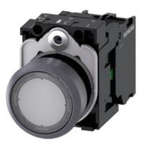
Illuminated pushbutton, 22 mm, round, plastic with metal front ring, clear, pushbutton, flat, momentary contact type, with holder, 1NO, LED module with integrated LED 230 V AC, screw terminal, with laser labeling, upper case and lower case, always upper case at beginning of line
