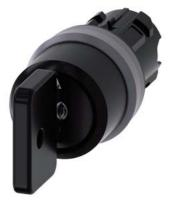
Key-operated switch O.M.R, 22 mm, round, plastic with metal front ring, lock number 73034, black, with 2 keys, 3 switch positions I>O<II, momentary contact type, actuating angle  $2x45^{\circ}$ , 10:30h/12h/13:30h, key removal O, Z=50-unit packaging
