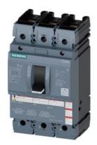
molded case switch 3VA5 UL frame 250 max. sh-circ breaking capacity 100kA @ 480 V 3-pole, line protection MCS110, In=250A without overload protection self-protection li=10 x In nut keeper kit on both sides
