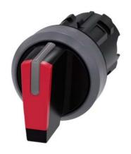
Selector switch, illuminable, 22 mm, round, plastic with metal front ring, red, selector switch, short, 3 switch positions I-O<II, left latching, right momentary contact type, actuating angle 2x45°, 10:30h/12h/13:30h, with laser labeling, upper case
