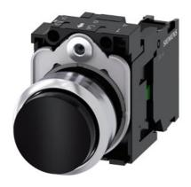
Pushbutton, 22 mm, round, metal, shiny, black, pushbutton, raised, momentary contact type, with holder, 1 NO, screw terminal, with laser labeling, upper case and lower case, always upper case at the beginning of the word
