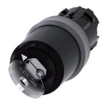
Key-operated switch IKON, 22 mm, round, plastic with metal front ring, lock number 360012K1, with 2 keys, 2 switch positions O<I, momentary contact type, Actuating angle 45°, 10:30h/12h, key removal O, Z=50-unit packaging
