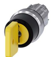
Key-operated switch O.M.R, 22 mm, round, metal, shiny, lock number 73033, yellow, with 2 keys, 3 switch positions I>O<II, momentary contact on the left, latching on the right, actuating angle 2x45°, 10:30h/12h/13:30h, Key removal II, with laser labeling, lower case
