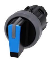
Selector switch, illuminable, 22 mm, round, plastic with metal front ring, blue, selector switch, short, 3 switch positions I>O<II, momentary contact on the left, latching on the right, actuating angle  $2x45^\circ$ , 10:30h/12h/13:30h, with laser labeling, upper case and lower case, always upper case at the beginning of the word
