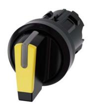
Selector switch, illuminable, 22 mm, round, plastic, yellow, selector switch, short, 3 switch positions I>O<II, momentary contact on the left, latching on the right, actuating angle  $2x45^{\circ}$ , 10:30h/12h/13:30h, with laser labeling, lower case
