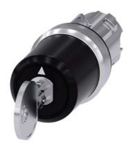
Key-operated switch BKS, 22 mm, round, metal, shiny, lock number S1, with 2 keys, 3 switch positions I>O<II, momentary contact on the left, latching on the right, actuating angle 2x45°, 10:30h/12h/13:30h, key removal O, with laser labeling, upper case and lower case, always upper case at beginning of line
