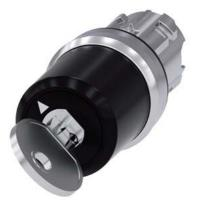
key-operated switch Siemens, 22 mm, round, metal, shiny, lock no. LSG1, with 2 keys, 2 switch positions O-I, latching, actuating angle 90°, 10:30h/13:30h, key removal O+I, Z=50-unit packaging
