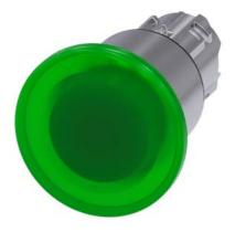
Illuminated mushroom pushbutton, 22 mm, round, metal, shiny, green, 40 mm, 3 switch positions, latches after pushing in, unlatches by pull-to-unlatch mechanism to center position, after pulling out the button Retraction to center position, with laser labeling, symbol number according to, ISO 7000 or IEC 60417
