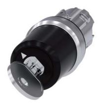
Key-operated switch BKS, 22 mm, round, metal, shiny, Lock No. E2 (VW), without key, 2 switch positions O-I, latching, actuating angle 90°, 10:30h/13:30h, key removal O+I, with laser labeling, upper case and lower case, always upper case at beginning of line
