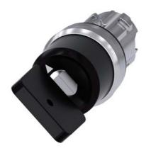
key-operated switch Siemens, 22 mm, round, metal, shiny, lock no. VL5, with 2 keys, 2 switch positions O<I, momentary contact type, actuating angle 45°, 10:30h/12h, key removal O, with laser labeling, upper case and lower case, always upper case at beginning of line
