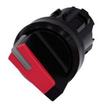
Selector switch, illuminable, 22 mm, round, plastic, red, selector switch, short, 2 switch positions O-I, latching, actuating angle 90°, 10:30h/13:30h, with laser labeling, upper case and lower case, always upper case at beginning of line
