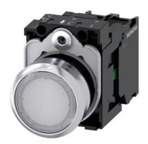
Illuminated pushbutton, 22 mm, round, Metal, shiny, white, pushbutton, flat, momentary contact type, with holder, 1NO, LED module with integrated LED 230 V AC, screw terminal, with laser labeling, upper case
