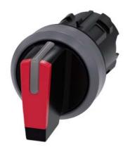
Selector switch, illuminable, 22 mm, round, plastic with metal front ring, red, selector switch, short, 3 switch positions I-O-II, latching, actuating angle 2x45°, 10:30h/12h/13:30h, with laser labeling, inscription or symbol Customer-specific selection with SIRIUS ACT configurator (CIN)
