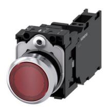
Illuminated pushbutton, 22 mm, round, metal, shiny, red, pushbutton, flat, momentary contact type, with holder, 1 NO+1 NC, LED module with integrated LED 110 V AC, spring-type terminal, with laser labeling, inscription or symbol Customer-specific selection with SIRIUS ACT configurator (CIN)
