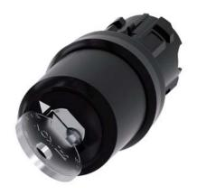
Key-operated switch IKON, 22 mm, round, plastic, lock number 360012K1, with 2 keys, 2 switch positions O-I, latching, actuating angle  $90^\circ$ , 10:30h/13:30h, Key removal O+I Z=50-unit packaging
