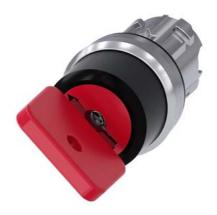
Key-operated switch O.M.R, 22 mm, round, metal, shiny, lock number 73037, red, with 2 keys, 2 switch positions O<I, momentary contact type, Actuating angle 45°, 10:30h/12h, key removal O, with laser labeling, upper case and lower case, always upper case at beginning of line
