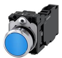
Pushbutton, 22 mm, round, metal, shiny, blue, pushbutton, flat, momentary contact type, 1 NO+1 NC, screw terminal, with laser labeling, inscription or symbol Customer-specific selection with SIRIUS ACT configurator (CIN)
