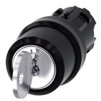
RONIS key-operated switch, 22 mm, round, plastic, lock number SB30, with 2 keys, 3 switch positions I>O<II, momentary contact type, actuating angle 2x45°, 10:30h/12h/13:30h, key removal O, possible special locks: SB31, 421, 455, with laser labeling, lower case
