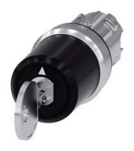
key-operated switch Siemens, 22 mm, round, metal, shiny, lock number SSG10, with 2 keys, 3 switch positions I-O-II, latching, actuating angle  $2x45^{\circ}$ , 10:30h/12h/13:30h, key removal I+II, with laser labeling, upper case
