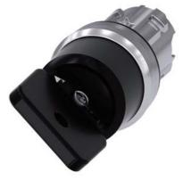
Key-operated switch O.M.R, 22 mm, round, metal, shiny, lock number 73034, black, with 2 keys, 2 switch positions O-I, latching, actuating angle 90°, 10:30h/13:30h, key removal I, with laser labeling, upper case and lower case, always upper case at beginning of line
