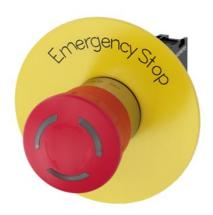
EMERGENCY STOP mushroom pushbutton, illuminable, 22 mm, round, metal, shiny, red, 40 mm, positive latching, acc. to EN ISO 13850, rotate-to-unlatch, with yellow washer, inscription: EMERGENCY STOP, with holder, 1 NC, 1 NC, LED module with integrated LED, 24-240 V AC/DC, red, screw terminal
