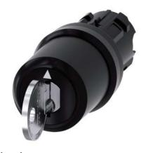
Key-operated switch IKON, 22 mm, round, plastic, lock number 360012K1, with 2 keys, 3 switch positions I-O<II, left latching, right momentary contact type, actuating angle 2x45°, 10:30h/12h/13:30h, key removal O+I, with laser labeling, inscription or symbol Customer-specific selection with SIRIUS ACT configurator (CIN)
