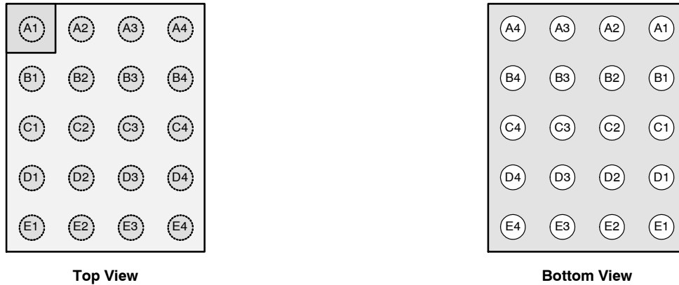
Figure 3. WLCSP-20 Pin Assignments
