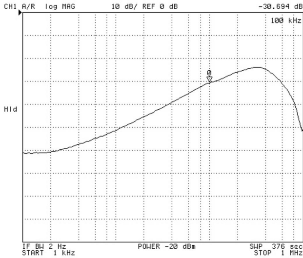
Figure 19. LDO1 PSRR vs. Frequency, V_{OUT1} = 1.2\text{ V} , I_{OUT1} = 150\text{ mA}
