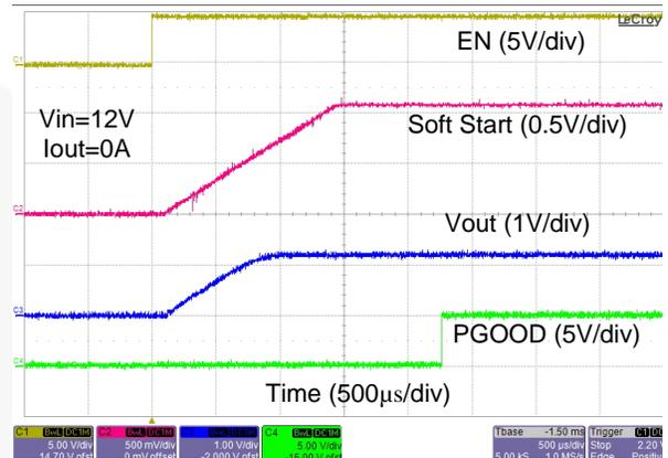
Figure 12. Startup Waveforms with 0 A Load Current
