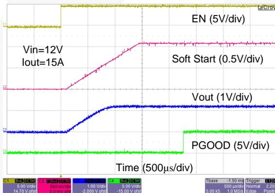
Figure 13. Startup Waveforms with 15 A Load Current
