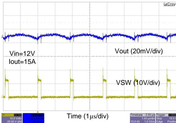
Figure 17. Static Load Ripple at Full Load
