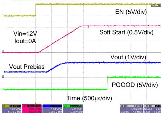
Figure 15. Startup Waveforms with Prebias Voltage on Output
