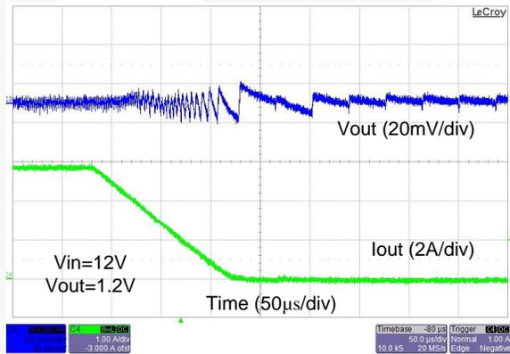
Figure 19. Transition from CCM to DCM Operation
