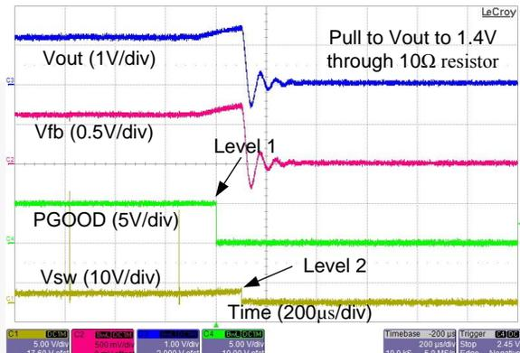
**Figure 23. Over-Voltage Protection Level 1 and Level 2**
