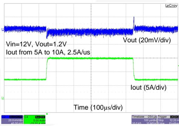
Figure 21. Load Transient from 50% to 100% Load Current
