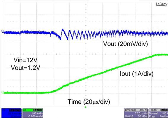
Figure 18. Transition from DCM to CCM Operation
