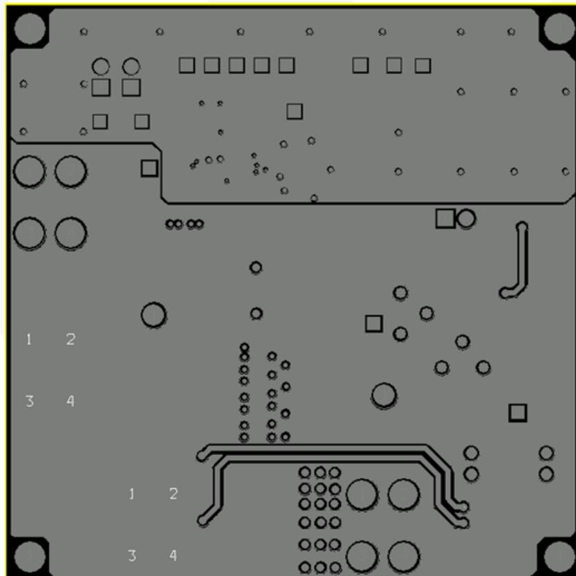
Figure 25. Evaluation Board Inner Layer 1 Copper
