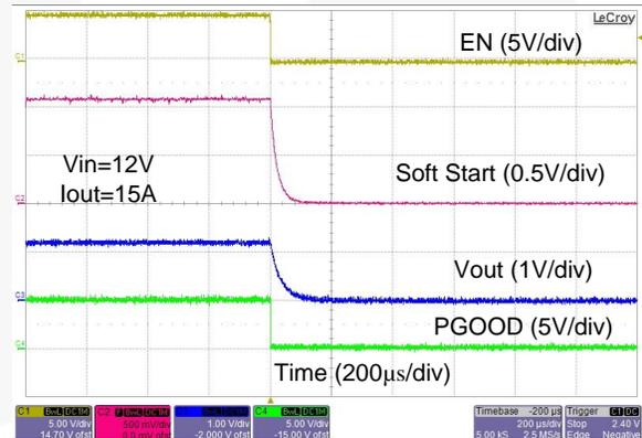
Figure 14. Shutdown Waveforms with 15 A Load Current
