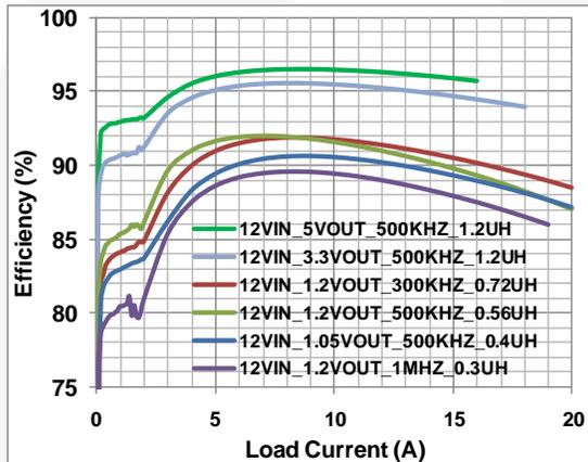
Figure 7. Efficiency vs. Load Current with  $V_{IN}=12\text{ V}$
