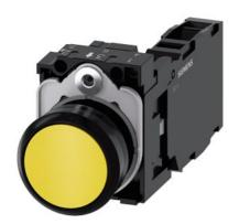
Pushbutton, 22 mm, round, plastic, yellow, pushbutton, flat, momentary contact type, with holder 1 NO+1 NC, screw terminal, with laser labeling, upper case
