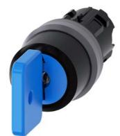
Key-operated switch O.M.R, 22 mm, round, plastic with metal front ring, lock number 73038, blue, with 2 keys, 3 switch positions I-O-II, latching, actuating angle 2x45°, 10:30h/12h/13:30h, key removal O, with laser labeling, lower case
