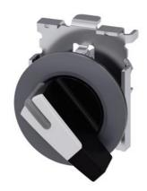
Selector switch, illuminable, 30 mm, round, Metal, matte, white, selector switch, long, front ring for flush installation, 2 switch positions O<I, momentary contact type, Actuating angle 45°, 10:30h/12h, with laser labeling, inscription or symbol Customer-specific selection with SIRIUS ACT configurator (CIN)
