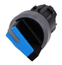
Selector switch, illuminable, 22 mm, round, plastic with metal front ring, blue, selector switch, short, 2 switch positions O-I, latching, actuating angle 90°, 10:30h/13:30h, with laser labeling, upper case and lower case, always upper case at the beginning of the word
