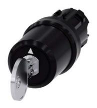
Key-operated switch BKS, 22 mm, round, plastic, lock number S1, with 2 keys, 3 switch positions I-O<II, left latching, right momentary contact type, actuating angle 2x45°, 10:30h/12h/13:30h, key removal O+I, with laser labeling, upper case and lower case, always upper case at the beginning of the word
