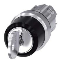
RONIS key-operated switch, 22 mm, round, metal, shiny, lock number SB30, with 2 keys, 3 switch positions I-O<II, left latching, right momentary contact type, actuating angle 2x45°, 10:30h/12h/13:30h, key removal O, possible special locks: SB31, 421, 455, with laser labeling, upper case and lower case, always upper case at the beginning of the word
