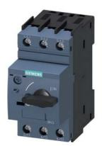
Special type Circuit breaker size S00 for motor protection, CLASS 10 A-release 1.8...2.5 A N-release 33 A screw terminal Standard switching capacity Ambient temperature -50  $^\circ$ C 500 switching cycles
