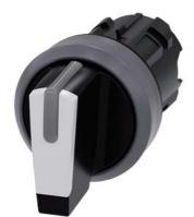
Selector switch, illuminable, 22 mm, round, plastic with metal front ring, white, selector switch, short, 3 switch positions I>O<II, momentary contact on the left, latching on the right, actuating angle  $2x45^{\circ}$ , 10:30h/12h/13:30h, with laser labeling, upper case and lower case, always upper case at the beginning of the word
