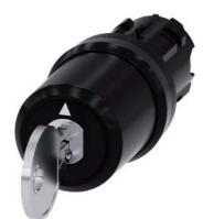
key-operated switch Siemens, 22 mm, round, plastic, lock number SSG10, with 2 keys, 3 switch positions I-O-II, latching, actuating angle 2x45°, 10:30h/12h/13:30h, key removal O, with laser labeling, lower case
