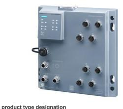
SCALANCE XP208EEC, managed IE switch with railway approval IEC 62443-4-2 certified; (EN 50155, EN 45545); 8x 10/100 Mbit/s M12 ports, IP65, LED diagnostics, error signaling contact, redundant power supply, PROFINET IO device, network management, can be operated in redundant ring, dust caps, including electronic manual on CD-ROM, C-plug optional.
