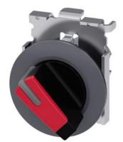
Selector switch, illuminable, 30 mm, round, Metal, matte, red, selector switch, short, front ring for flush installation, 2 switch positions O<I, momentary contact type, Actuating angle 45°, 10:30h/12h, Z=50-unit packaging
