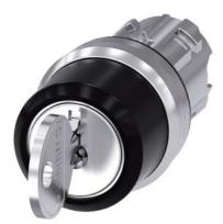
RONIS key-operated switch, 22 mm, round, metal, shiny, lock number SB30, with 2 keys, 3 switch positions I-O-II, latching, actuating angle 2x45°, 10:30h/12h/13:30h, Key removal I+II, possible special locks: SB31, 421, 455, with laser labeling, lower case
